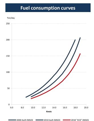
ECO 2018-built VLCC vessels are significantly more fuel efficient than older tonnage
